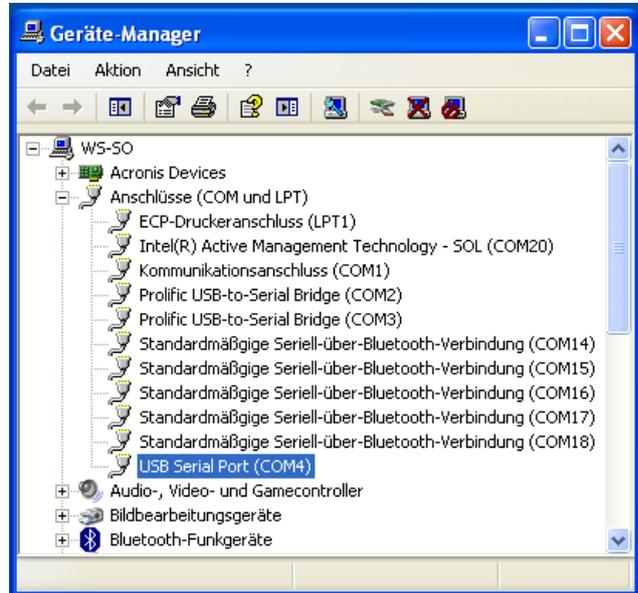
**COMx set must be between COM1....COM9 and it should be ensured that there is no double occupancy of the interfaces.**
