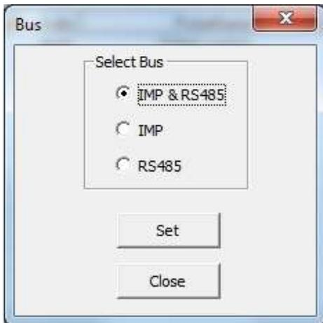
The serial interface inside the SONO probe can be selected to IMP-Bus or RS485. Due to very robust behavior it is recommended to select the IMP-Bus.
